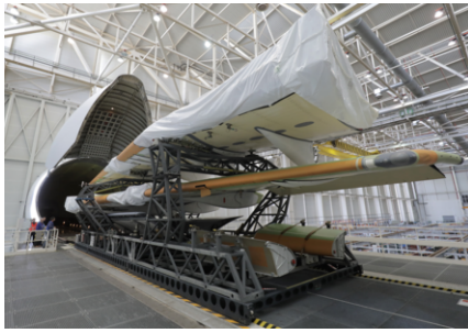
(a) Unloading/Loading of a wing from/to a Beluga aircraft. The part stands on a jig which goes itself on a mobile rack to transfer the unloaded/loaded part to/from the outside rack system.
