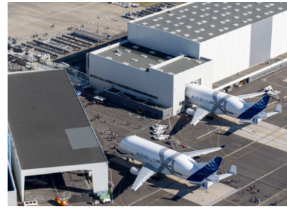
(b) Beluga hangar and outside rack system (top left corner of the picture) where aircraft jigs and their held parts are temporarily stored before being sent to the factory.
